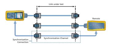
Figure 3. Pair-to-pair Alien FEXT measurements. The main and remote units are plugged into different cabling links at opposite ends of the bundle under test. A spare channel in this bundle connects the synchronization modules plugged into each of the testers to allow the testers to perform all of the pair-to-pair FEXT measurements between the wire pairs of two selected cabling links.
