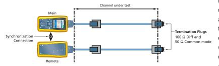
Figure 2. Pair-to-pair Alien NEXT measurements. The main and remote units are sitting side-by-side at one end of the cabling bundle under test. These units are plugged into different cables. A standard patch cord connects the synchronization modules plugged into each of the testers to allow the testers to perform all of the pair-to-pair NEXT measurements between the wire pairs of two selected cabling links.
